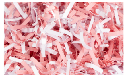
2 x 15 mm particles of security level P-5 according to DIN 66399 (ISO/IEC 21964)
